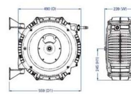
Construction: Enclosed reel – Heavy duty UPVC plastic
