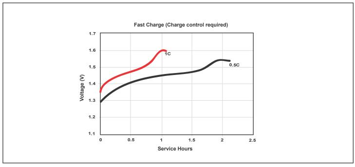
Product can be charged on most nickel metal hydride (NiMH) chargers utilizing standard dV, dV/dt, time and temperature dynamic charge termination methods. Duracell brand chargers are recommended for best results.
