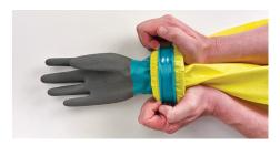
Step 7 - Using both hands push the AlphaTec\* ribbed green collar further up the sleeve until tightly locked in position. Ensure outer ring is tightened as far as possible to provide a secure fit.
